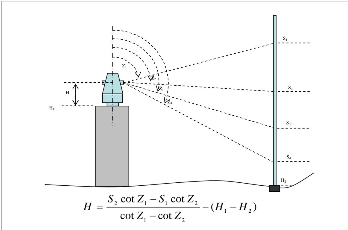
**Figure 7:** Total station instrument heighting technique, where  $S_n$  are staff readings;  $Z_n$  are zenith angles (Rueger & Brunner, 1981).
