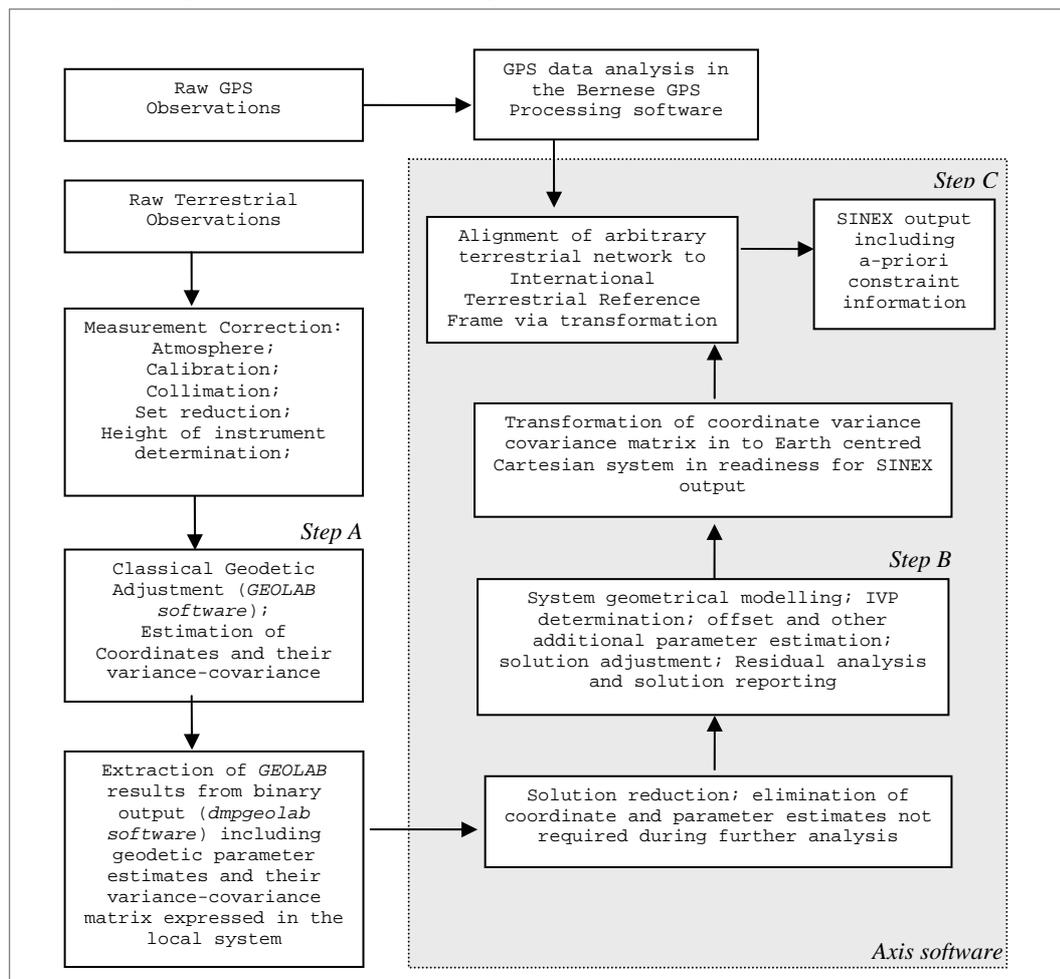
Figure 9: Analysis process for the reduction of local survey data.
