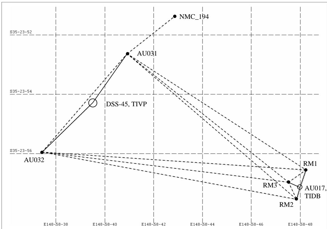
**Figure 3:** Tidbinbilla 2007 terrestrial geodetic network. Terrestrial observations between stations are shown as inter-connecting lines.
