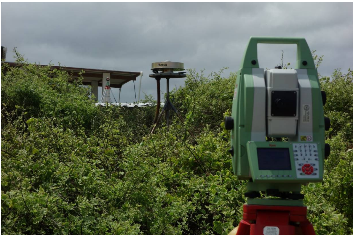
Total station on point 16 with GLPS and point 17 in background
