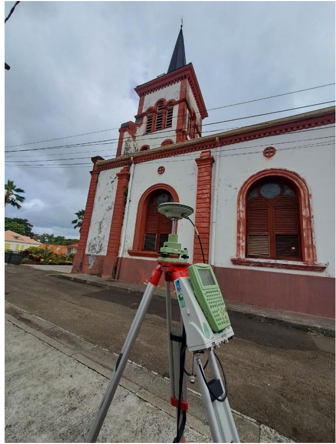
GNSS antenna on station 502 and point 2000
