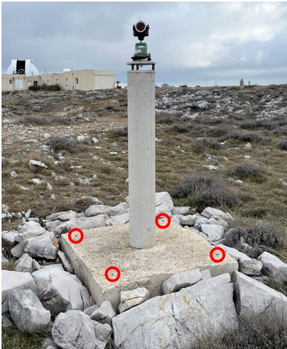
Pillar n°4 with a reflector; benchmarks are in the red circle
