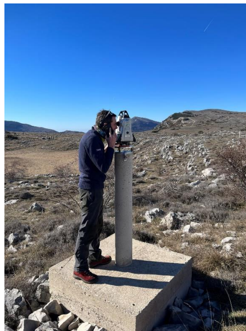
Total station on pillar n°3
