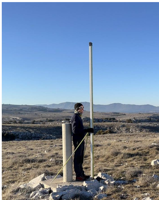
Levelling on benchmark, pillar n°3
