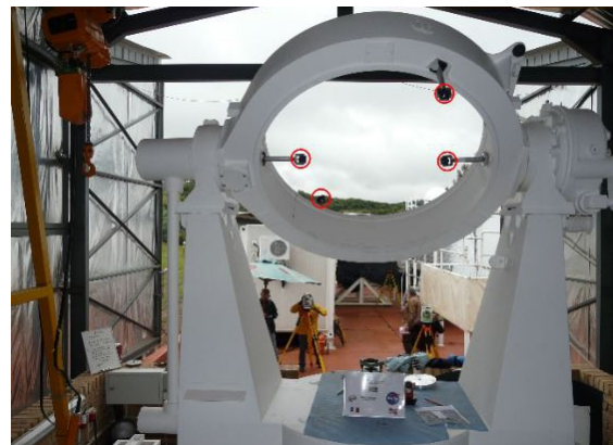
Prisms for horizontal axis determination
