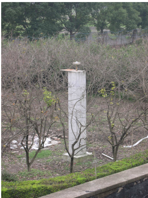
Choke Ring antenna of EGNOS GPS station
