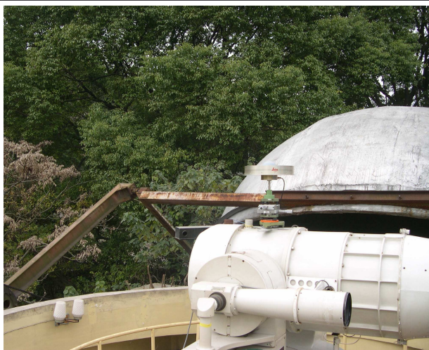
Choke ring antenna set up on the translation stage
