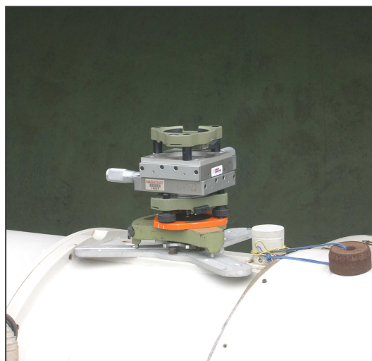
Platform with translation stage on vertical axis
